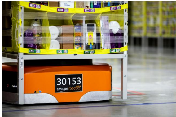
Figure 11 Amazon Robotics robots delivering movable shelves to the picker (Source: Amazon)
